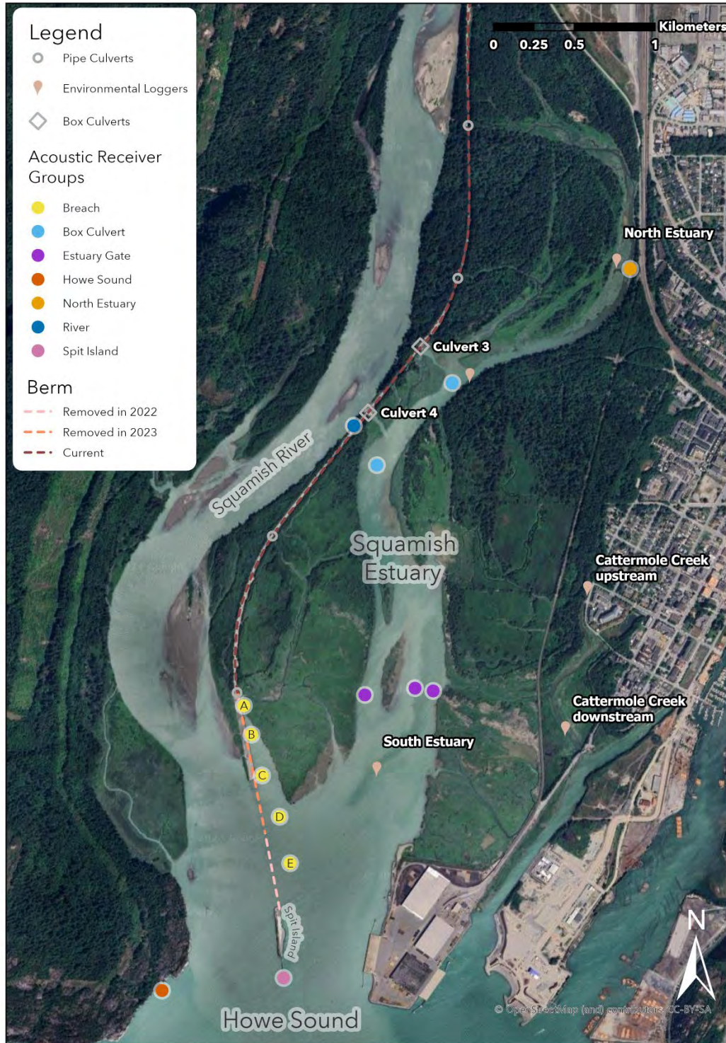
Figure 2 Map of the acoustic receivers and environmental loggers in the Squamish River Watershed. Environmental loggers include dissolved oxygen, salinity, temperature, and depth sensors. Portions of the berm were removed in 2022 and 2023. The tip of the berm was not removed, creating Spit Island. Pipe culverts installed in the late 1990s - early 2000s and box culverts installed in 2019 and 2020 are also shown.
